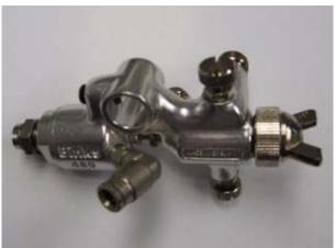
The customer wanted to reduce lubricant consumption and clean up the fluid application on their production tube bending operation. A system was designed that provides electronic timing and sequencing of the spray system. A pneumatically triggered, air atomizing spray head was added to provide precise control of the spray pattern. Fluid and air pressure regulators allow finite control of the fluid delivery and spray characteristics.
